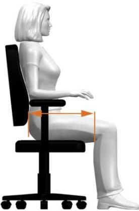
Figure 4. Seat Depth (horizontal distance between the buttock and the back of the knee)
