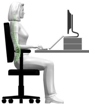
Figure 7. Example of an appropriate torso-to-thigh angle
