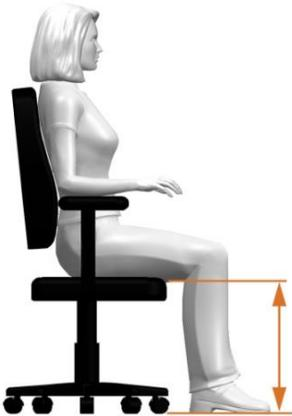
Figure 3. Seat Height (vertical distance between floor and back of the knee)
