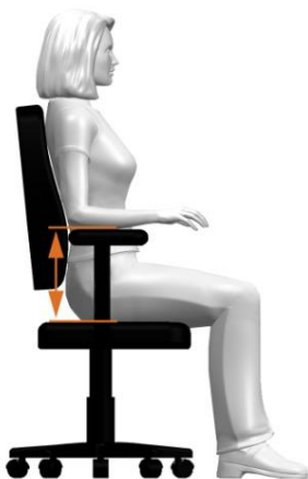
Figure 8. Armrest height (vertical distance between the seat pan height and the seated elbow height)
