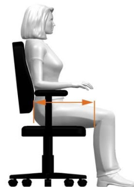
Figure 4. Seat Depth (horizontal distance between the buttock and the back of the knee)
